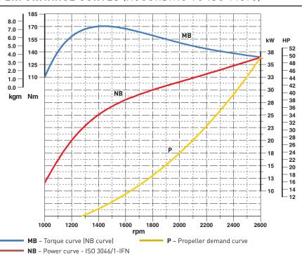
Power ratings refer to engines equipped with air filter, standard muffler, after running-in period at ambient conditions of +25°C, relative humidity 30% and 1 bar. Power levels drop by 1% every 100 m altitude and by 2% every 5°C above +25°C.
